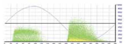
➤ Phase-resolved display of a partial discharge at 50 Hz
