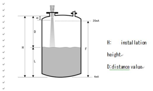
An integrated temperature sensor compensates for changes in the velocity of sound caused by temperature changes. Calibration Enter the empty distance H and the span F to calibrate the device. +
