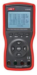
**Short review UNI-T UTM 1267B (267B).** Designed for measuring three-phase AC voltage and current, phase angles between voltages, currents or both, frequency, phase sequence, active, reactive and apparent power, power factor, sum of current vector.
