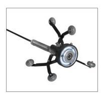
The Type "B" Adjustable Skid, for the D46/SL, is used for larger diameter pipes in lines from 8 to 15 inches in diameter. The Type "B" Skid is made of aluminum with stainless steel hardware and polyurethane wheels.
