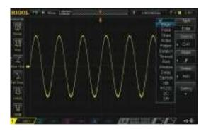
Built-in dual-channel 25 MHz source (DS1XX4Z-S Plus)
