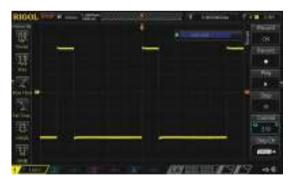
Serial bus trigger and decoding functions (RS232/ UART, I2C, SPI)
