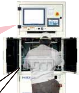
The system reads the number of the pin contacted with the probe.
