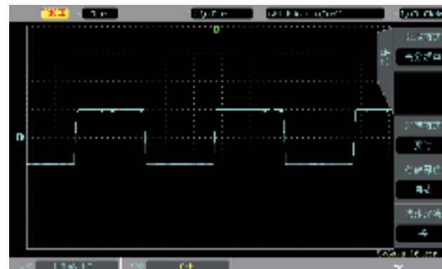
High Resolution mode to minimize noise from small signal
