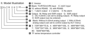
Please note input signal type when choosing model. 1st type: TC/RTD/mV/Rt; 2nd type: mA/V. There is only one 4 ~ 20mA output for the whole series meters. In size of 6, 8, 9, when the relay output,ssr output exsist together with 4-20mA output. "I" used to distinguish. Such as IR, IQ ect. But for 3, 4, 7 size, it does have this kind of model.
