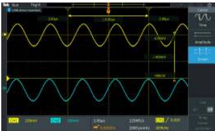
The cursor readouts are presented on the waveform display. Cursors can be used to measure time and amplitude.
