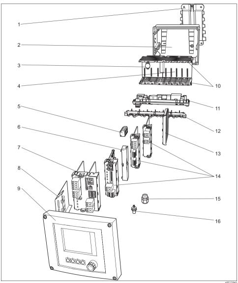
Abb. 2: Spare parts: You can find the names of spare parts and their order numbers in the following table.
