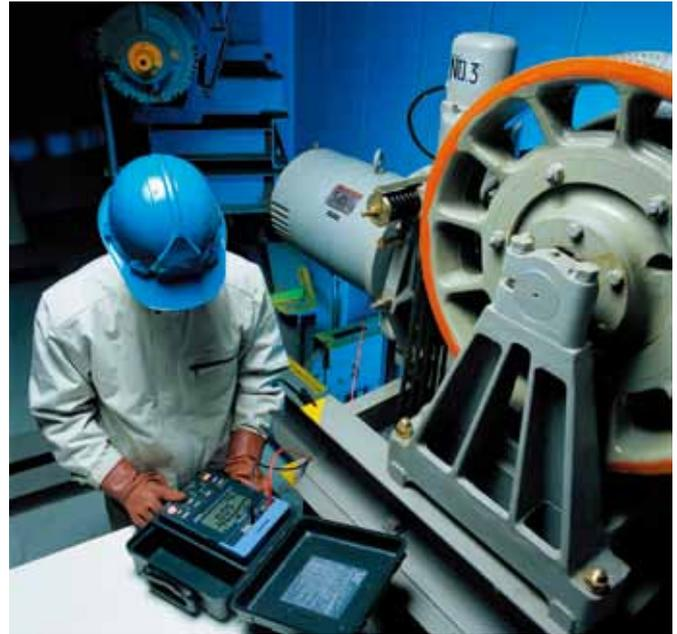
safety regulations for category IV measurements (600 V). A shutter mechanism prevents simultaneous use of measurement terminals and other terminals. Other safety features include a voltage measurement function, high-voltage warning indicator, and auto discharge function.
