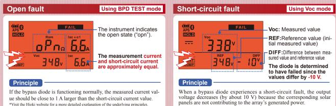
panels are not contributing to the array's generated power. By detecting this difference, it is possible to detect bypass diode short-circuit faults and cell string losses.
