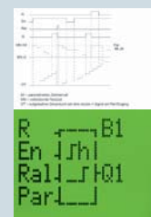
Operating hours counter
