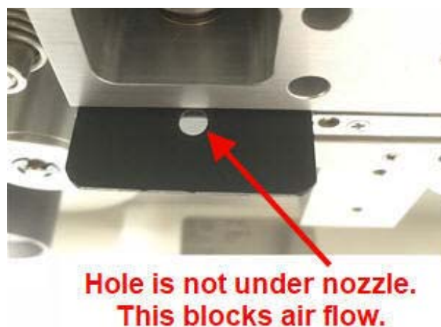
Figure 5-4 Nozzle Seal Tool with Solid Side Under the Nozzle
