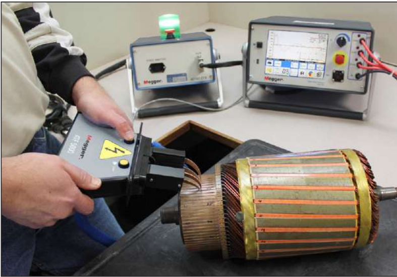
Performing armature tests is easy with the ATF5000 and Baker ZTX low-impedance component test accessories
