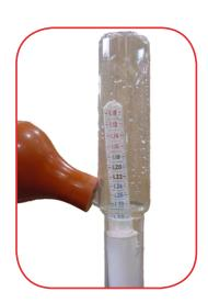
A scale inside the stem makes it easy to read specific gravity.
