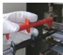
For clamping around the target busbar
