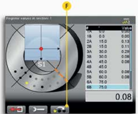
Display screen for section measurement method. Point 6 on outer circle to be measured. It is possible to skip any measurement point (F), in this example point 4B.
