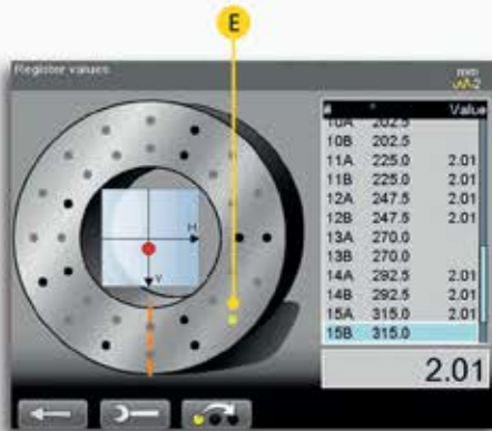
The point to be measured is indicated in the image. It is also possible to see from the display screen whether the laser beam hits the detector.
