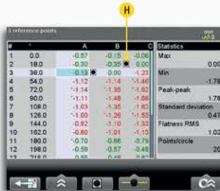
Result table with reference points marked (H). Red values are out of tolerance.
