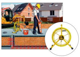
Using a fiberglass locating cable allows you to reliably find the exact position of sewers and PE ductworks. Depending on the connection to the Easyloc TX transmitter, either the entire route can be located or just the tip of the cable. The fiberglass locating cable is available in a large variety of lengths.
