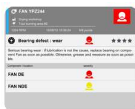
Detailed information on a defect with identified location
