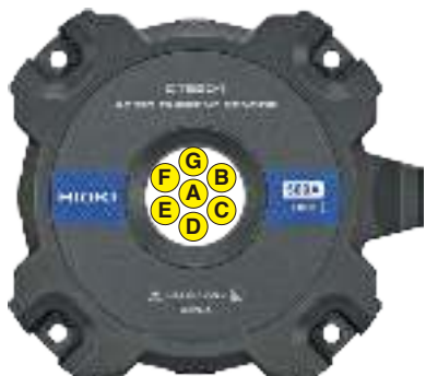
When using a sensor designed with the effects of conductor position, measured values are not affected when the conductor's position changes.
