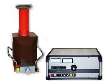
Compact, maintenance free, cast-resin highvoltage transformers
