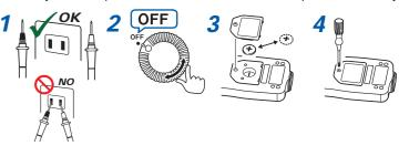
Do not turn the adjustment screw inside the battery case. Doing so will cause the instrument to report abnormal measured values.
