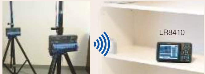
Data is sent wirelessly from measurement units to the LR410.
