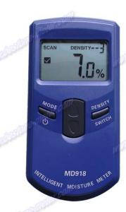
result will be discplayed in its clear LCD in an instant. Different types of wood correction value of are already set in this handy meter. Specifically made for professionals in wood industries such as wood crafts, wood facilities, wood furniture, wood flooring, wood products, etc.
