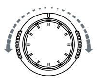
This knob provides quick Adjust/Locate function for numerical parameters with relatively large settable range. Turn clockwise (counterclockwise) to increase (reduce) the value. The inner knob is used for fine adjustment and the outer knob for coarse adjustment.
