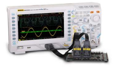
Figure 6 To Connect the Logic Probe
