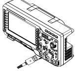
Figure 5 To Connect the Passive Probe
