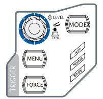
**MODE**: press this key to switch the trigger mode to **Auto**, **Normal** or **Single** and the corresponding state backlight of the current trigger mode would be illuminated.
