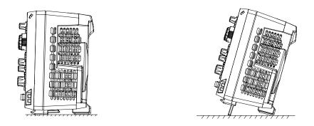
Figure 3 To Adjust the Supporting Legs
