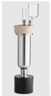
Fully assembled Test Cell in the assembly stand with glass fill and riser funnels.
