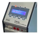
Set your automatic ramp (slope) with up to 0.1C per minute rate. The PTB 1200 will store for you the contact open and closed. No need for any additional mustimeter.
