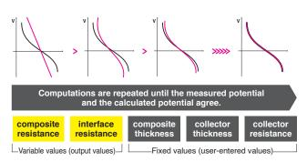
The calculated potential is computed while varying the variables.
