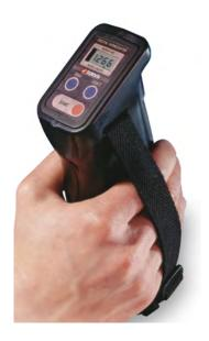
The SBS-2002 is lightweight, durable and easy to use, making it suitable for use in all industrial environments. Simply insert the nozzle into the battery and depress the finger pump which draws a few drops of sulfuric acid (H<sub>a</sub>SO<sub>a</sub>) through the tube. Within three seconds the measured refractive index is converted into a temperature-compensated specific gravity reading and then both the specific gravity and temperature are displayed.
