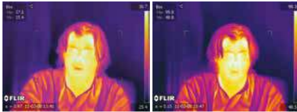
The thermal image on the left has the right emissivity settings for human skin (0.97) and the temperature reading shows the correct temperature (36.7 °C). For the thermal image on the right, the wrong emissivity was entered (0.15), leading to a false temperature reading (98.3 °C).
