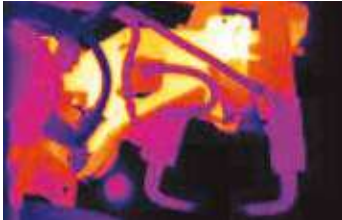
Hot spot in welding robot
