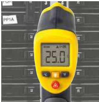
IR thermometer, temperature measurement in one spot
