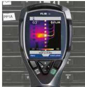
FLIR i3, temperature in 3,600 spots
