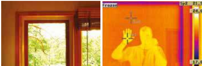
The window reflects thermal radiation, so to a thermal imaging camera the window acts as a mirror.
