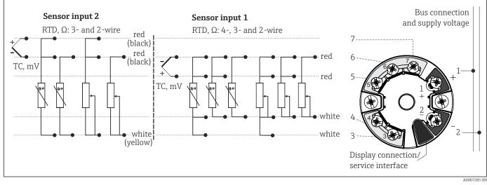
Assignment of terminal connections for head transmitter
