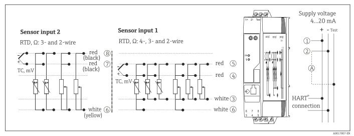
Assignment of terminal connections for DIN rail device
