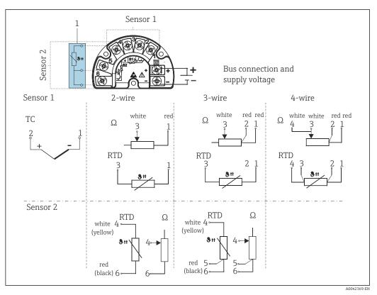
■ 5 Terminal assignment of the field mount housing with separate terminal compartment
