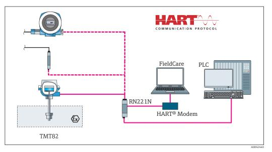
■ 2 Device architecture for HART<sup>®</sup> communication
