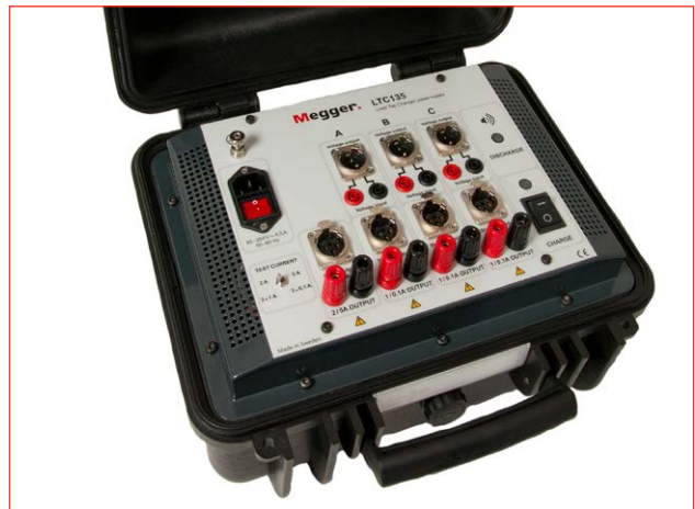
LTC135, Load Tap Changer power supply
