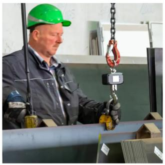
Force gage with a measuring range of 0 ... 1000 kg / Backlit LC display / Battery operation / Robust metal housing / "Hold", "Tare" and "MAX" functions / Various mass units / Optionally with ISO calibration certificate
