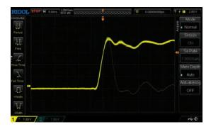
UltraVision: waveform recording and playback functions
