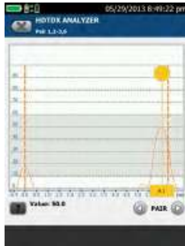
High Definition Time Domain Cross talk (HTDIX) shows the far end connection is clearly the issue
