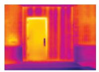
**Air leakage:** Identify sources of energy loss due to improperly installed or worn seals on windows and doors.
