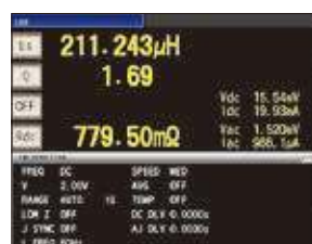
L, Q and Rdc continuous measurement screen
