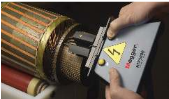
The ATF5000 armature test accessory makes testing armatures with many coils and commutator segments easy and fast
