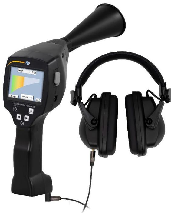
The new PCE-LDC 15 leak detector is used wherever gases can escape from leaks in piping systems, for instance in compressed air, gas and vacuum systems in industrial areas as well as door seals. The operating frequency of the leakage tester is 40 kHz ( $\pm 2$  kHz).
