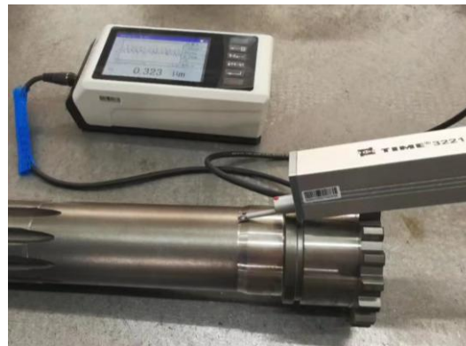
Measure conical surface
